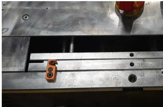
Illustration 81: Safeguard of the ejector system (with ejectors under sliders)
