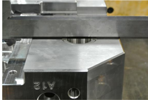
Illustration 14: Flush-mounted guide bush
