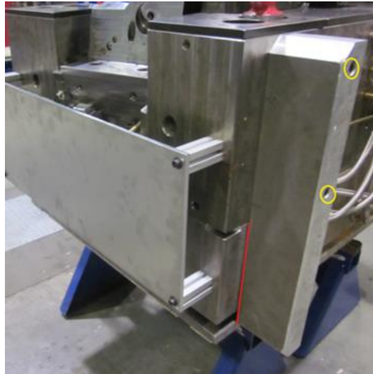
Illustration 26: mold standing bar
